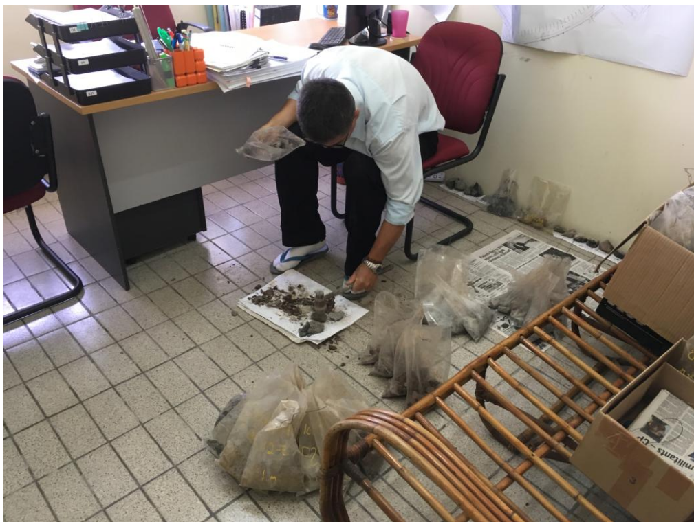
Photo 18: J6- Checking the Rock's Hardness and Record the Description
