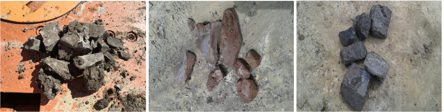
Photo 17: Bedrock Samples for Confirmation (Shale and Sandstone)
